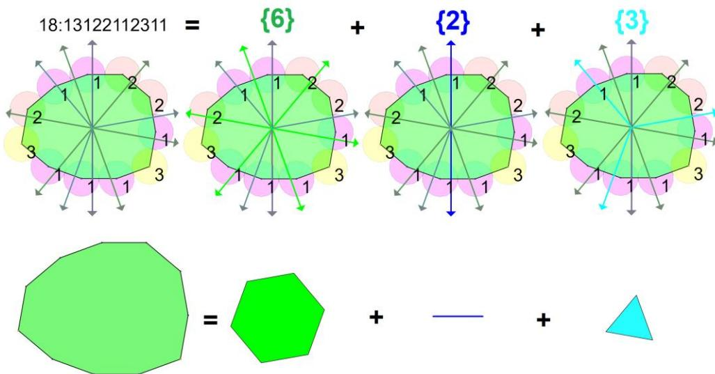
Figure 14 Decomposition of an asymmetric 18-tile
